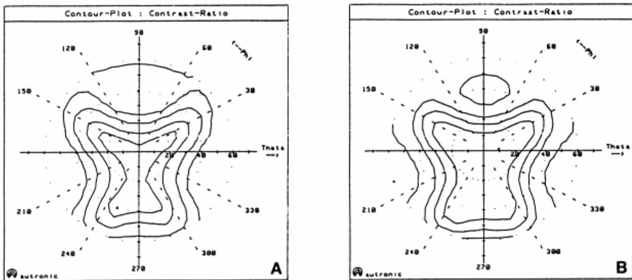
Figure 5: Contrast of a TN-LCD measured in transmissive mode of operation (left) and under multi-directional diffuse illumination (right). The intrinsic directional characteristics of the contrast of the LCD which is obvious in the transmissive mode can only be reproduced under multi-directional diffuse illumination in the reflective mode of operation [from 10].
