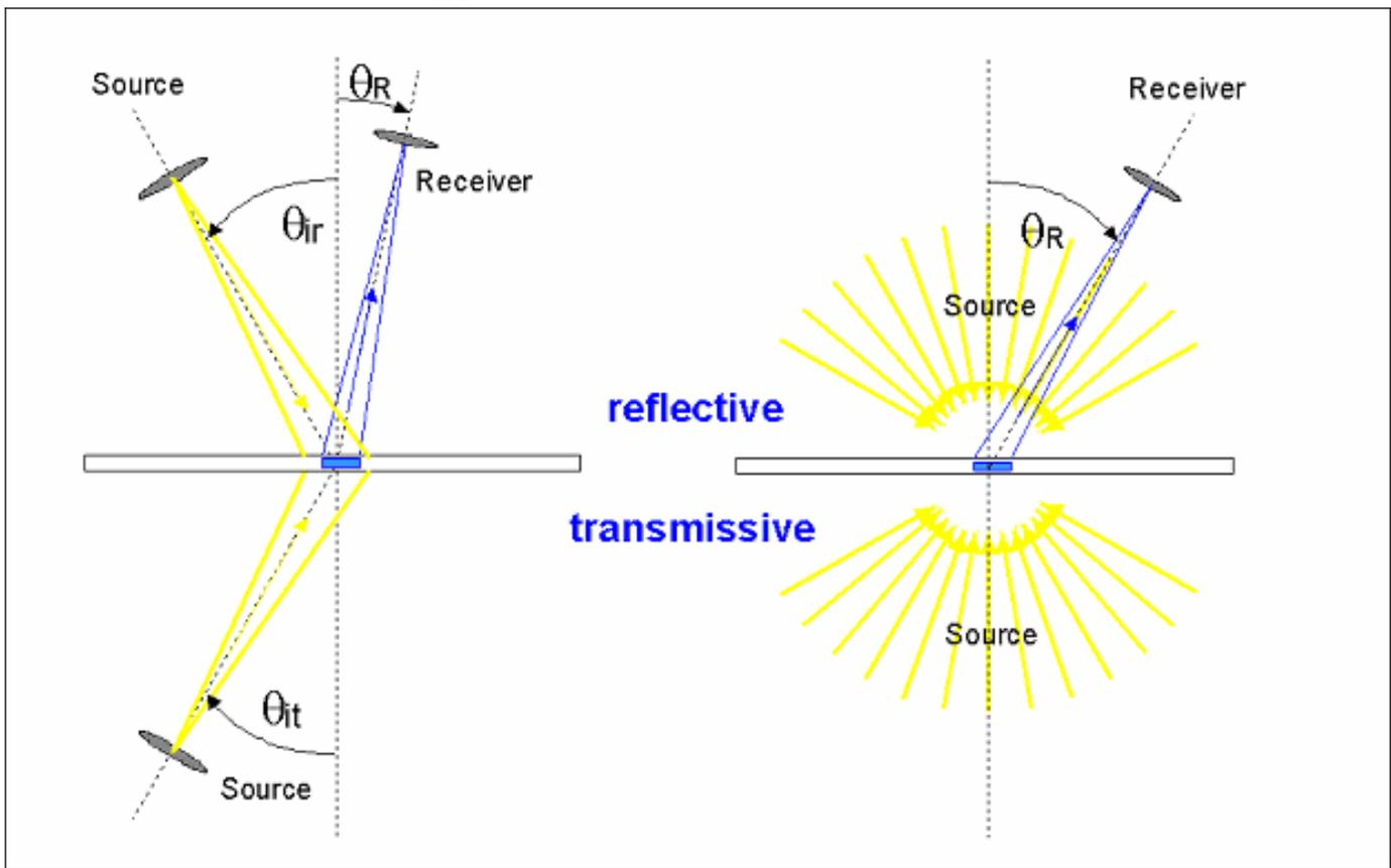
Figure 1: Two arrangements for measuring the electro-optical performance of LCDs. Directional illumination (DI, left) and multi-directional diffuse illumination (MI, right) for transmissive and reflective mode of LCD operation.
