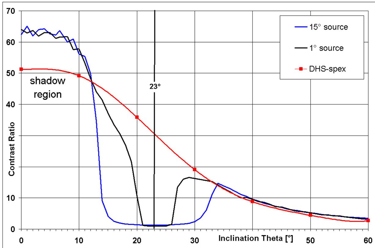
Figure 4: Contrast (luminance ratio) vs. angle of inclination of a reflective TN-LCD measured under directional illumination ( $1^\circ$  and  $15^\circ$  source) and multi-directional diffuse illumination (spex: specular components excluded). Data and illustration from [9].
