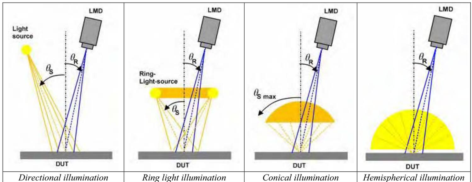
Figure 6: Illustration of the four basic illumination schemes introduced in the proposal for the metrology standard for reflective LCDs, IEC 61747-6-2 under discussion. Only the arrangement with hemispherical illumination can be used for directional scanning of the viewing cone of the DUT.
