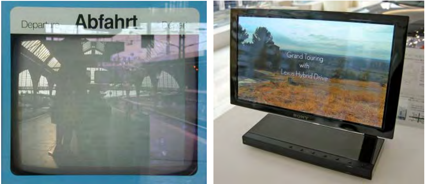
Figure 1 on the left: Railway timetable shown on a CRT display with an anti-reflection coated vandal-proof cover glass, exhibiting reflections from ambient light sources (sky, lamps). The visual information can only be read (though with very low contrast) in the regions with shadow. Figure 2 on the right: A modern shiny TV screen (2008), based on OLED technology, showing reflections of ambient light in the mirror-like display surface (source: http://commons.wikimedia.org/wiki/Image:Sony_OLED_TV_XEL-1.JPG )
