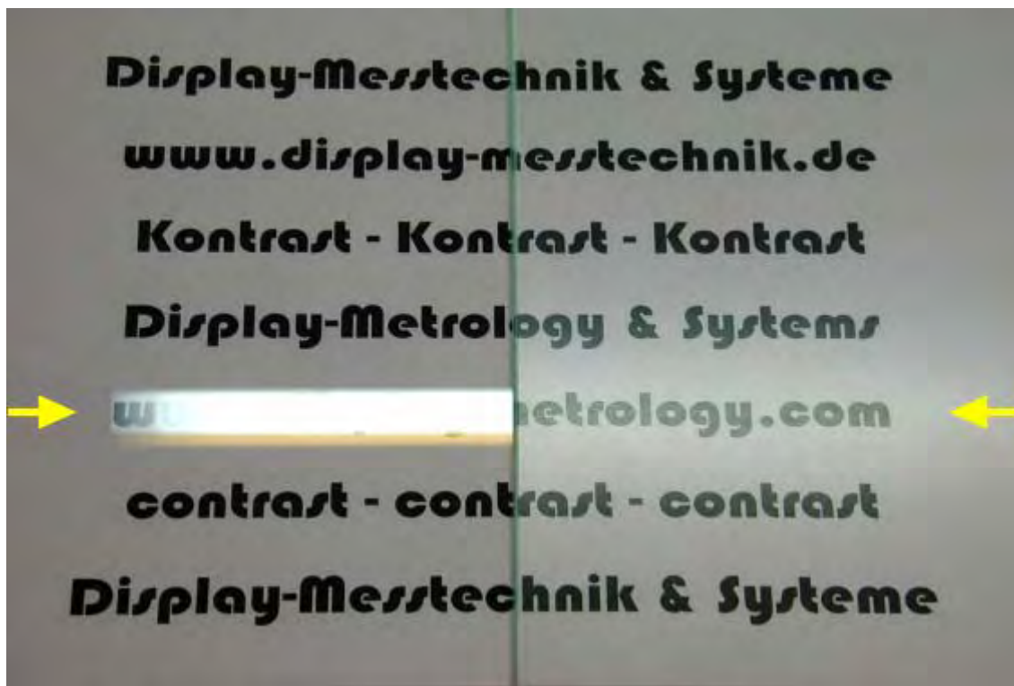
Figure 3: Visual information in the presence of reflections with glossy (left) and matte surface (right). The arrows indicate the position of the light source (fluorescent tube). While the light source is distinctly visible in the part of the display with the smooth surface (yellow arrow in the left half), it can only be noticed as a fuzzy area that is somewhat brighter than the surroundings (yellow arrow in the right half).
